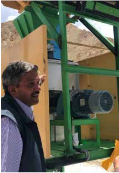
In-vessel composting machine
