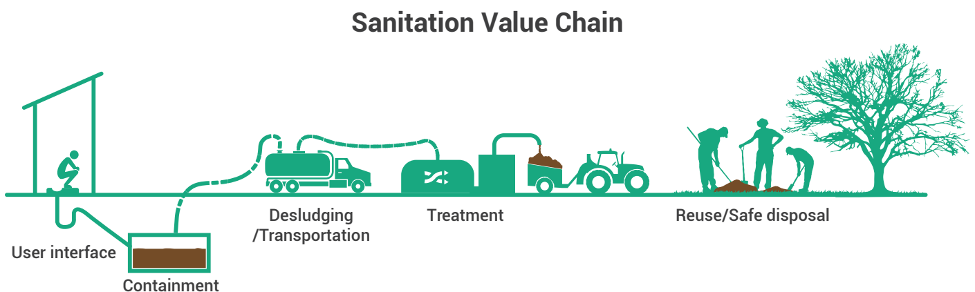
Figure 1: Flow diagram of Faecal Sludge Management
